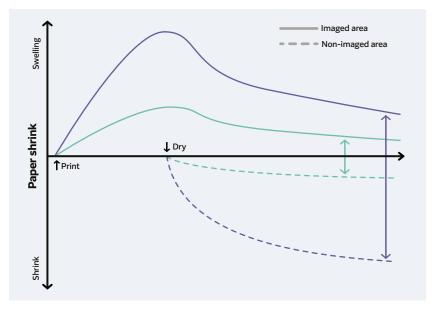
Stabilised paper, represented by the green line, swells and shrinks less as it carries less moisture overall from the start of printing the first side, to the end of drying the back side.
