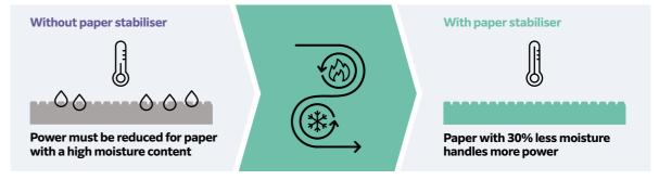
Many presses printing high resolution on coated stocks need to slow down to 50 metres per minute or less. When paper is stabilised on the Jet Press 1160CFG, lower moisture content means the paper surface can withstand more power and run at higher speeds.
